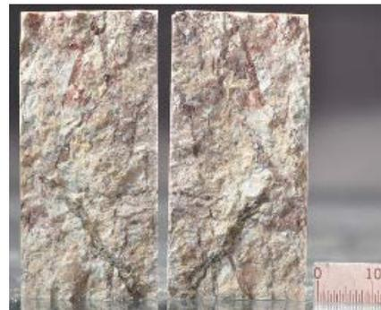
FIGURE 2: FRACTURED SUB-CORE BCH-03 4580 A WITH MM SCALE.
