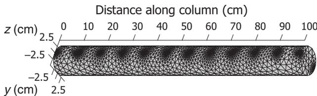
Figure 1. Image of column used for electrical forward modeling. The location of the 12 electrodes can be seen in the mesh; Wenner data were collected along these electrodes between neighboring electrodes. To create maps of electrical conductivity for this column, 1D transport simulations were converted to fluid electrical conductivity and then bulk electrical conductivity.
